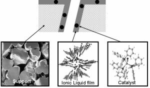
Figure 1: Schematic representation of a Supported Ionic Liquid (SILP) catalyst`
