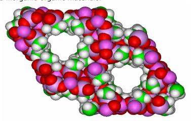
Molecular modelling is now being used to help determine the structure and properties of compounds like the AlMePO structure shown above. By careful design, these materials can be optimised for their potential applications.
