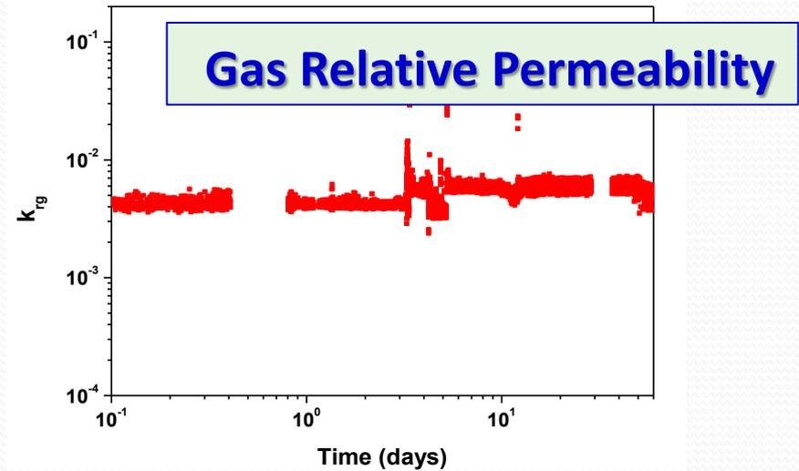
End (steady-state) gas permeability:  $k_{rg}^0(S_w = 0.93) = 0.005$
