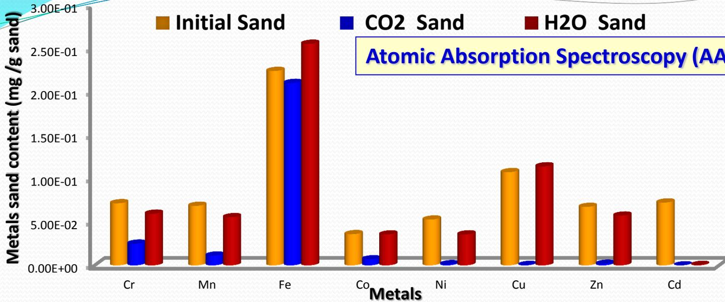
**Content of metals in the sand before and after the flow experiments**
